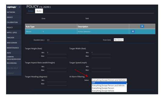
To enable AI, choose an option from the AI Alarm Filtering drop-down.
