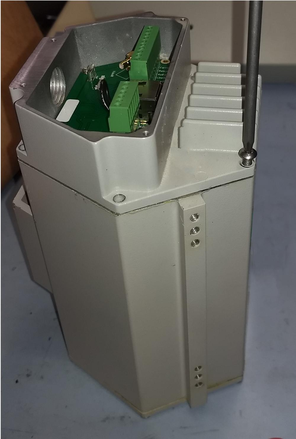
**15. Replace the backplate using the supplied (longer) 440 flathead, 1/2" screws.**
