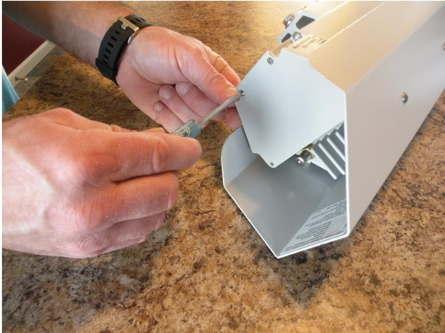
The back plate is held in place with screws which do not need to be removed entirely. Back out the screws maintaining forward pressure until you feel the threads disengage. The gasket will hold the screws in place while the back plate is removed.
