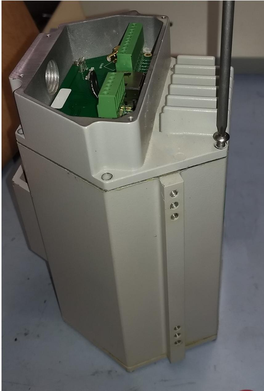
**5. Pull back assembly back to reveal the connectors.**
