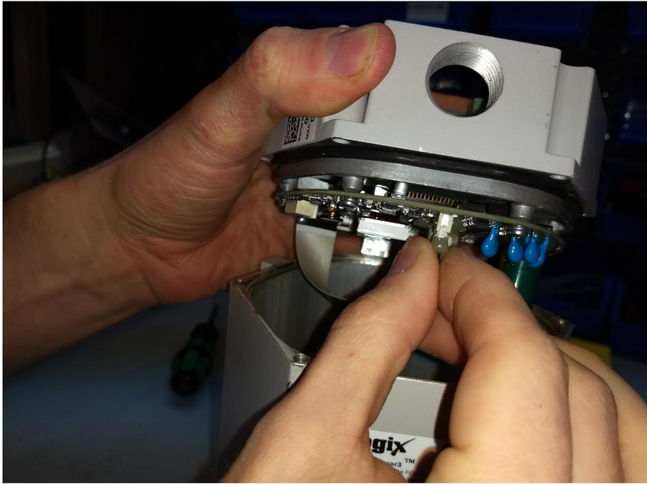
**14. Place back assembly on chassis and lightly turn six T15 or T20 screws to place. Then tighten all six in a cross pattern.**
