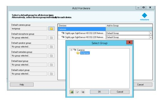
• Click Finish. A successfully added camera appears as shown. If you have a SightSensor HD, the visible and thermal sensors will be added as two cameras from the same IP address.
